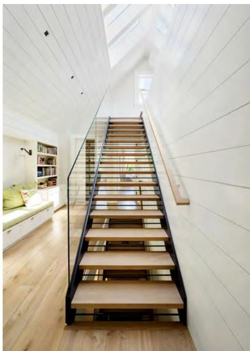
The new staircase at the center of the house is made from blackened steel and glass, and topped by skylights.
